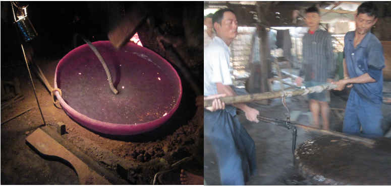
Figure 31: Starting to look like a gong; putting into water source: author
