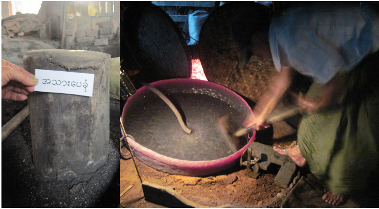
Figure 32: Wooden anvil; upright edge source: author
