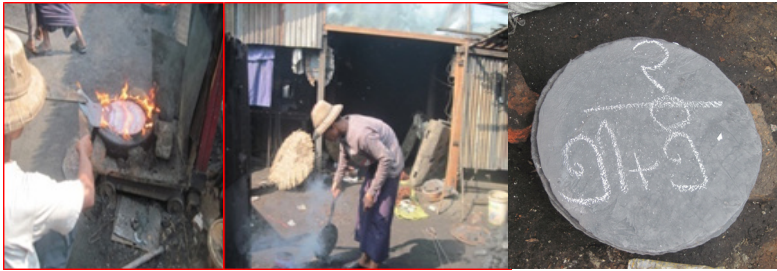
Figure 22: Removing impurities; molten figure; Myo-khe brass plate source: author
