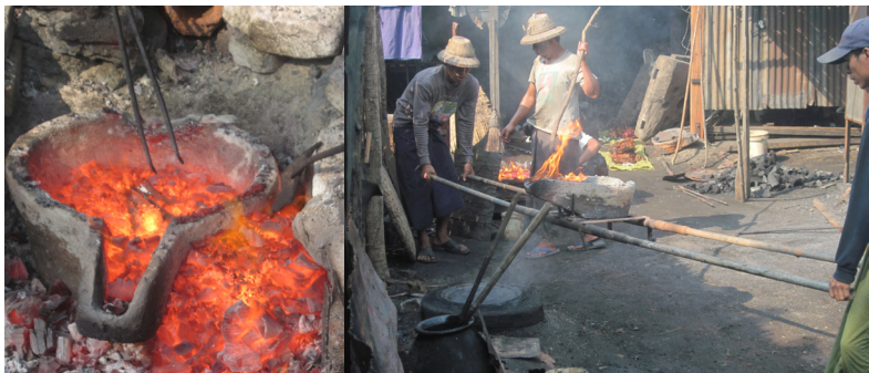
Figure 25: Lower pot; carrying molten brass source: author
