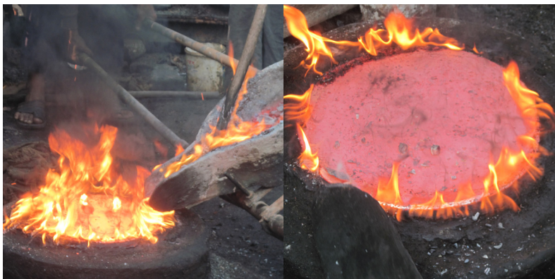
Figure 26: Rough cloth filter; Liquid flows into the mold source: author
