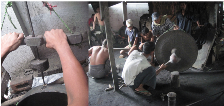
Figure 38: Drilling a hole in the gong; testing the sound source: author
