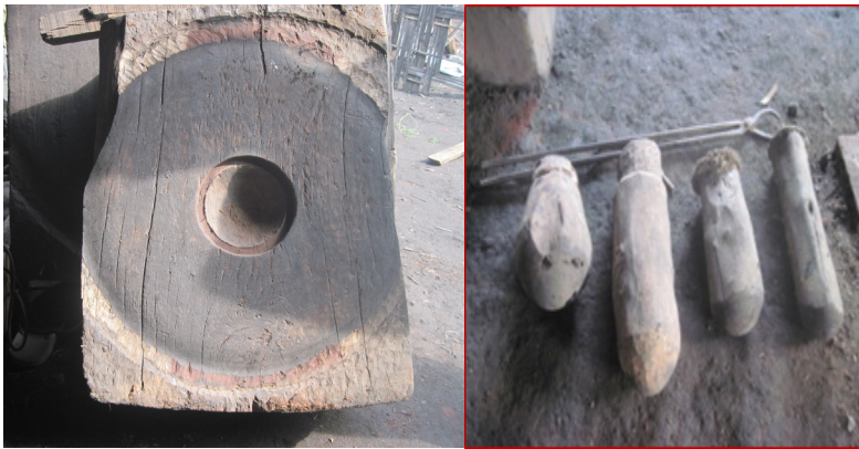
Figure 34: Wooden concave anvil; Wooden pestles source: author
