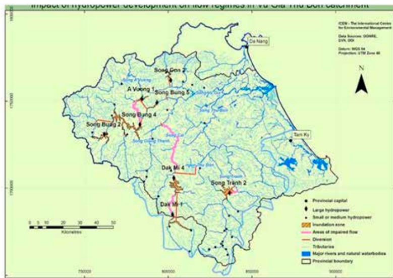
Figure 4.4 Master plan of cascade hydropower on Vu Gia-Thu Bon River Basin Basin Source: ICEM (2008), cited in CSRD (2014)
