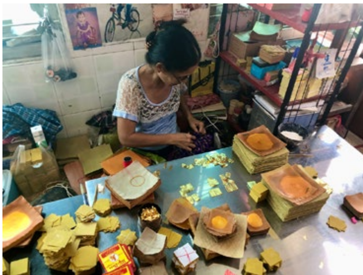
Figure 2.20 Assembling gold leaf packets (Htet Htet Khaing)
